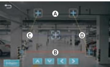
Make sure that (A) and (B) are horizontally parallel, and that (C) and (D) are the same length.
