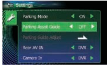
You can display parking guidelines to enable easier parking when you shift the gear to the reverse (R) position.
